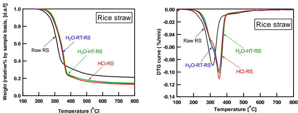
Figure 1. (a) TG curves and (b) DTG curves of washed and Raw-RS.
