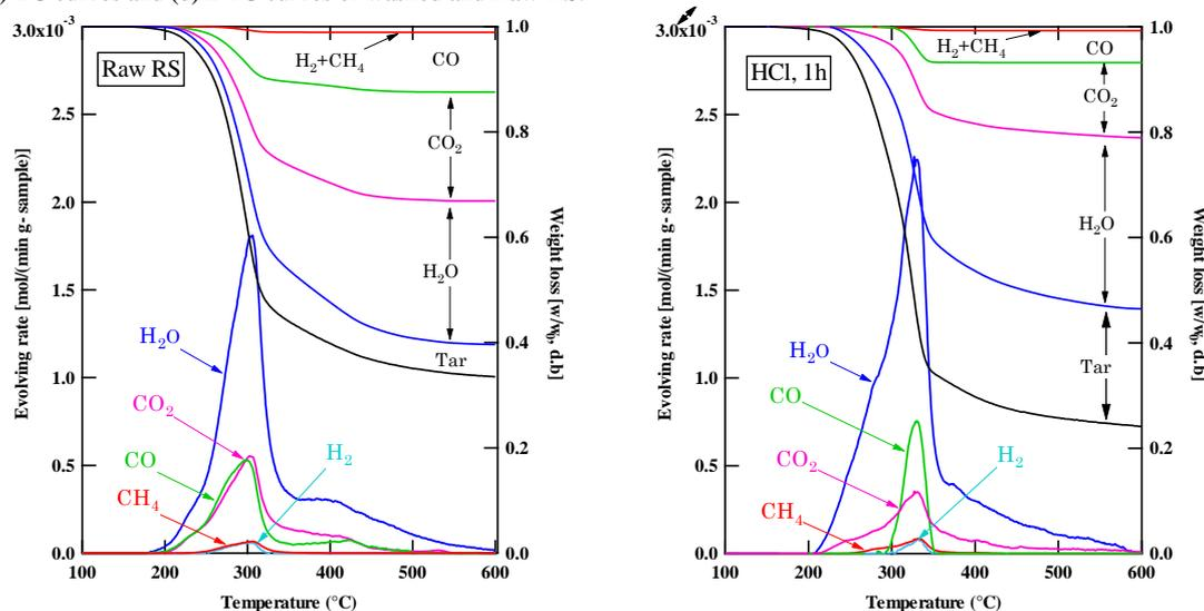
Figure 2. TG curve, gas formation rate and product distribution during the pyrolysis of raw of Raw-RS and HCl.
