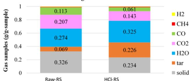
**Figure 3.** Product yield (H<sub>2</sub>, CH<sub>4</sub>, CO, CO<sub>2</sub>, H<sub>2</sub>O and tar) of Raw-RS and HCl-RS.
